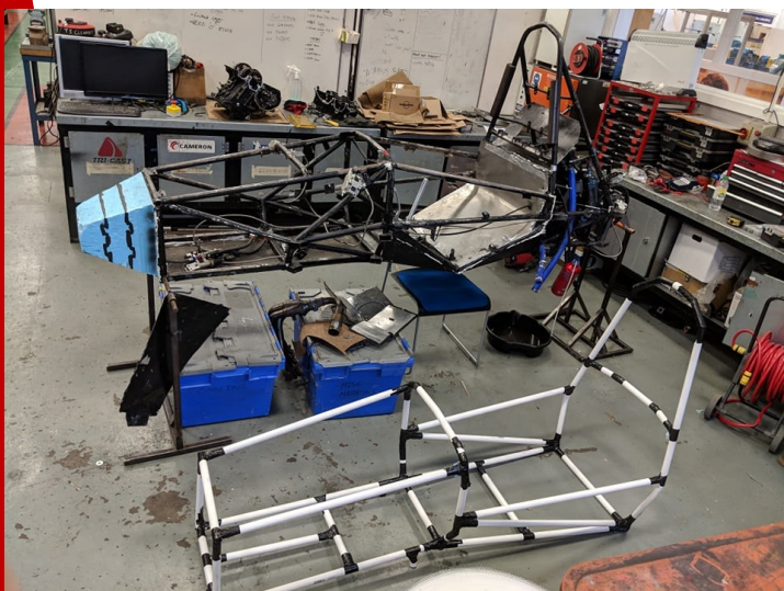
HARE 19 Mock up Chassis, compared with HARE 19 Chassis
