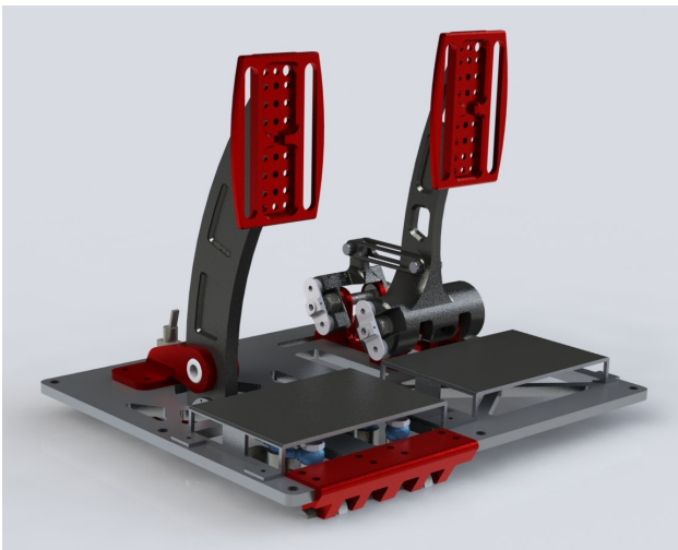
HARE 19 Pedal Box SolidWorks Render
